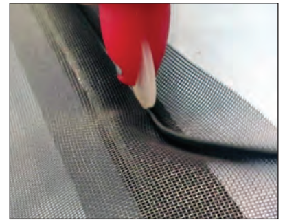
Spline rollers used to fit screen & spline into groove
